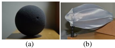
Figure 4. Photographs of wind shields used for the measurements: a) 180 mm spherical, and b) Windpac.
